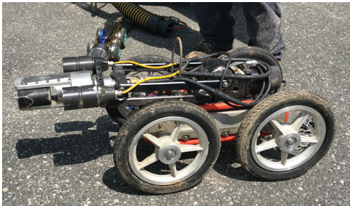
The mobile camera used to examine the inside of the pipe.
